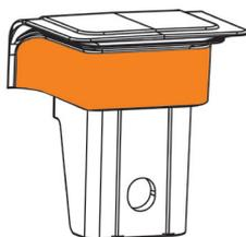
**For outdoor installation, cover the marked areas of the seal rubber plug with technical grease:**
