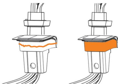
**For outdoor installation, cover the marked areas of the wiring harnesses with provided technical grease:**
